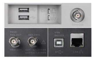
2 x USB 2.0 Host, 1 x USB 2.0 Device (USBTMC) 1 x 10M/10M LAN (VXI-11/Telnet/Socket) 1 x Auxiliary Output (Pass/Fail and Trigger Out)
